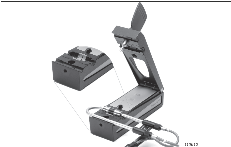
Fig. 2. The final calibrator. The probe is a 1/2" probe with a 12 mm spacer. The slit with the sound source is seen in the middle of the coupler cavity
